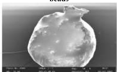
Fig 2. SEM photomicrograph of cross-sectional calcium alginate bead
