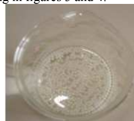
Fig 3. Calcium alginate beads (F-13) floating in (SGF) without pepsin in a beaker (top view).
