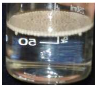
Fig 4. Calcium alginate beads (F-13) floating in (SGF) without pepsin in a beaker (side view).
