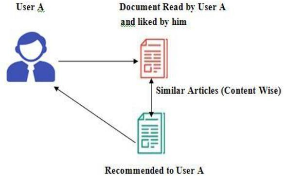
**Fig 2: Content based recommender system**
