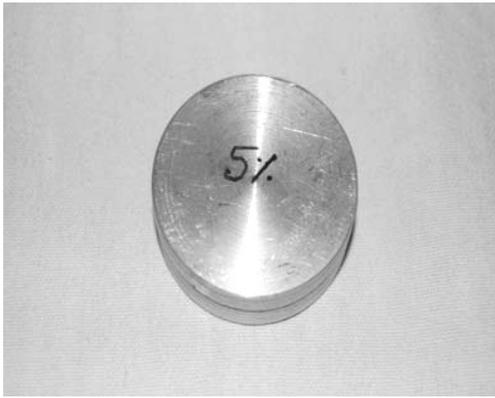
**Figure 1:** Specimen 5 % SiC with Aluminium
