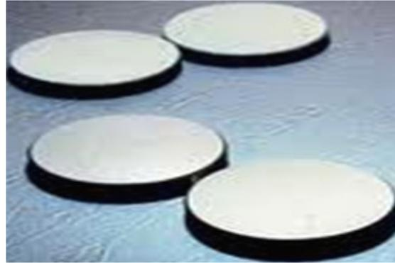
**Figure 2:** Samples of Aluminium-Silicon Carbide
