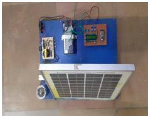
Fig.7: Hardware model for the developed battery monitoring system
