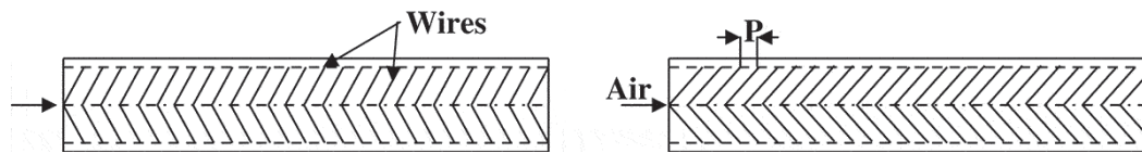
Fig. 14. V-shaped rib roughness
