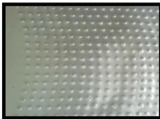
Fig. 21. Dimple shaped roughness arranged in angular arc shape
