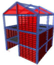
Figure 5 3D RC Infilled Frame with Link Element
