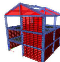
Figure 4 3D RC Infilled Frame with Gap Element
