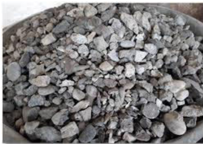
Fig. 3 Coarse Recycled Aggregate
