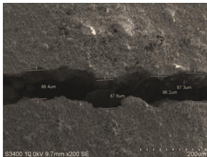
Figure.3. Depicts the propagation of cracks in concrete containing 2% PVA fibers at a strain of 2%.
