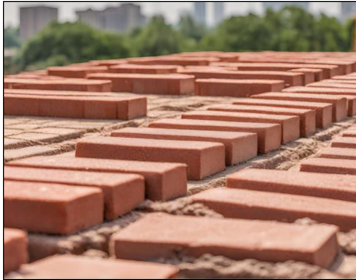
Figure 3: Natural drying of bricks
