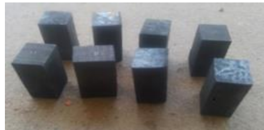
Figure 3. H13 steel samples after annealing
