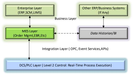
**Figure 1.** A simplified high-level concept of how MES integrates with enterprise systems (ERP, SCM, LIMS) while interfacing with the DCS or PLC-based Process Control System. This architecture underpins critical business drivers like resource optimization, real-time visibility, and compliance.
