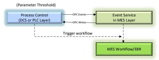
**Figure 2.** In an event-driven approach, DCS automatically triggers MES workflows upon detecting real-time process conditions (e.g., crossing a parameter threshold). This model is highly effective for time-to-market and efficiency drivers, enabling dynamic responsiveness.
