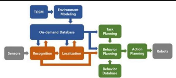
**Figure 1:** The proposed framework consists of semantic modeling framework (SMF) (blue blocks), semantic information processing (SIP) module (orange blocks), and semantic autonomous navigation (SAN) module (green blocks).
