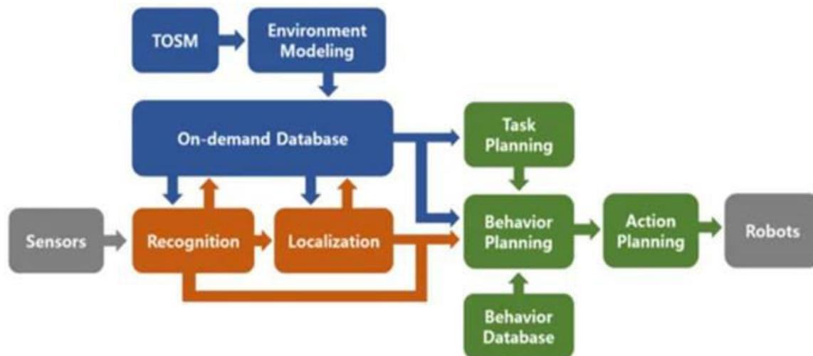
**Figure 1:** The proposed framework consists of semantic modeling framework (SMF) (blue blocks), semantic information processing (SIP) module (orange blocks), and semantic autonomous navigation (SAN) module (green blocks).
