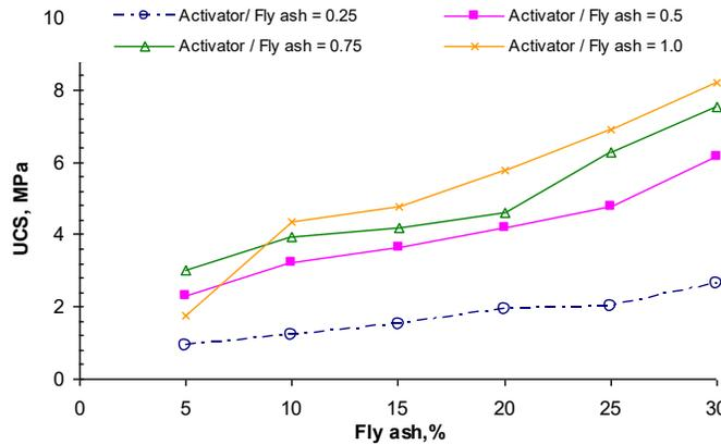
Figure 4: Variation of UCS with the fly ash content considering different activator ratios
