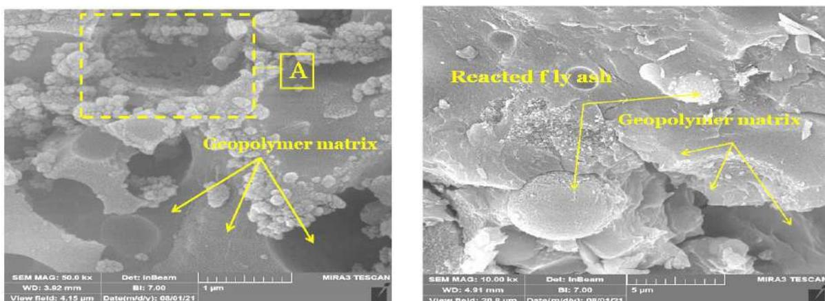
Figure 6. SEM of geopolymerized soil (Fly ash=20%, Ac/FA=0.5)
