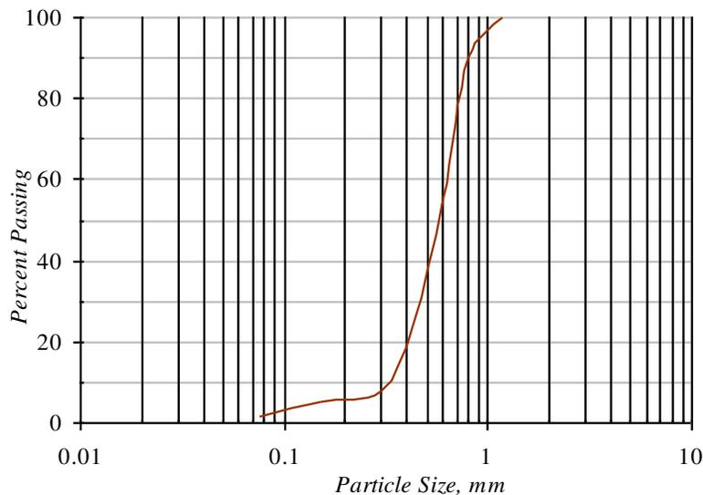
**Figure 1:** Grain size distribution of the used sand
