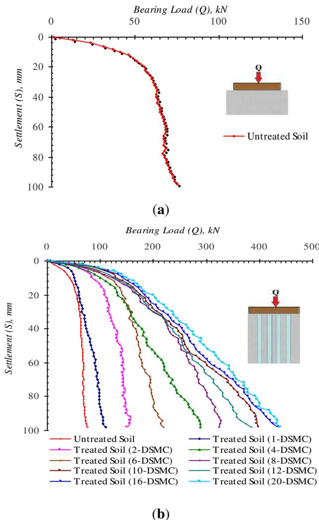
**Figure 5.** Relationship between the bearing load and the settlement of: (a) untreated soil; (b) soil treated with different numbers of DSM columns
