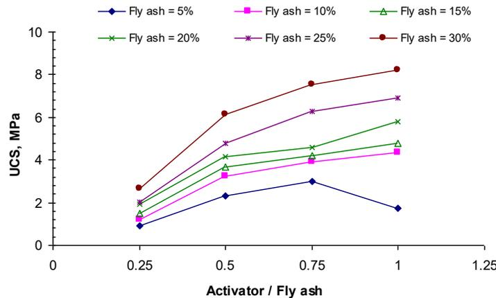
Figure 4: Variation of UCS with activator ratios considering different fly ash contents
