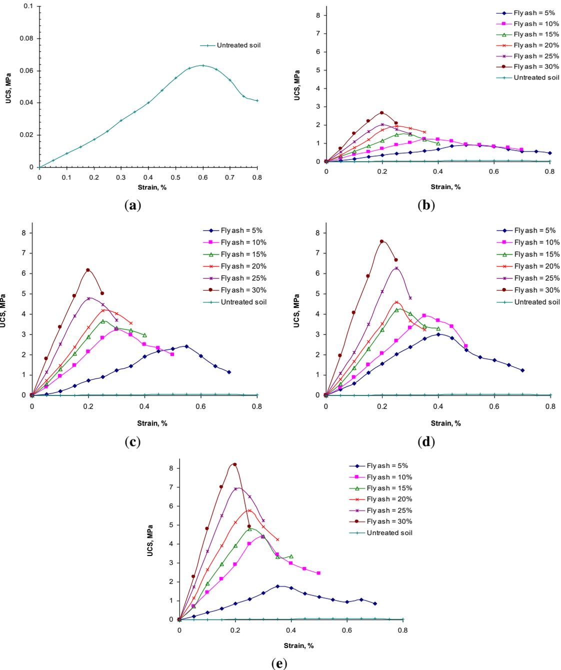
**Figure 3.** Stress-strain relationships of geopolymerized sand considering different fly ash content at : (a) untreated soil; (b) AC/FA=0.25; (c) AC/FA=0.5; (d) AC/FA=0.75; (e) AC/FA=1.0.
