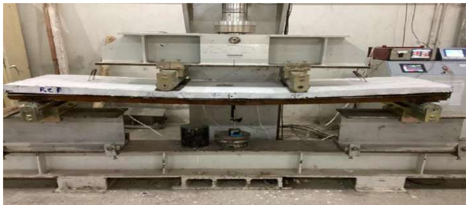
Figure 4: Specimen result of reference slab case study
