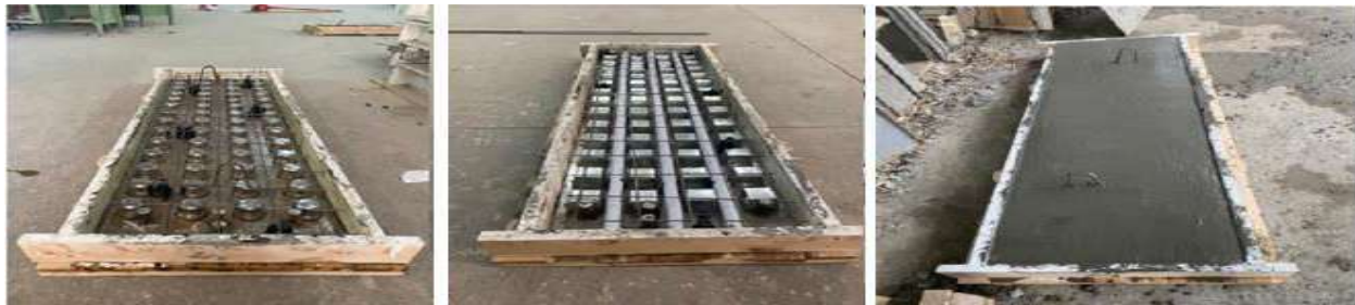
Figure 3: Developing and casting the mold.
