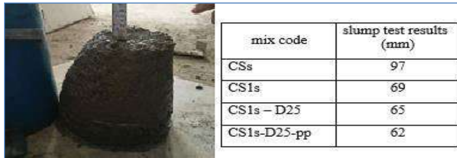
Figure 2: slump test
