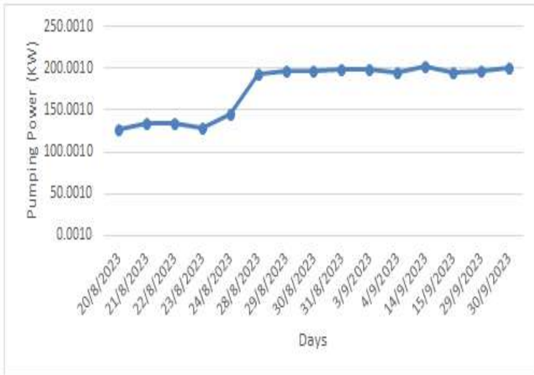
Fig. 18: variation of Pumping Power (KW) with The Days for EAHE system.
