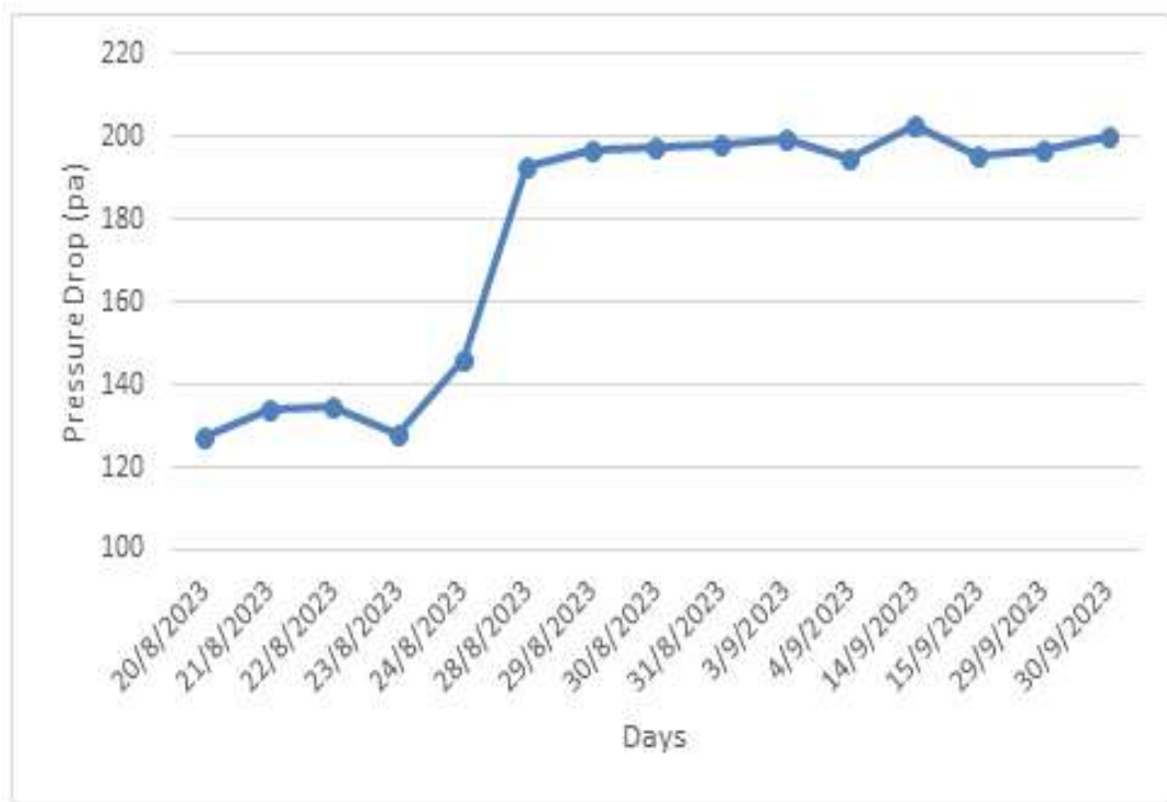
Fig. 17: variation of Pressure Drop (pa) with The Days for EAHE system.
