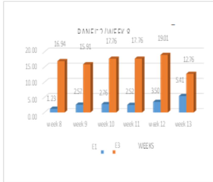
Figure 5: Percentage loss in the output performance ratio of panels A and C compared to panel A
