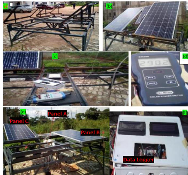
Figure 3: Experimental set-up (a-b) 0 to 40 degrees tilted platform(c)Temperature and humidity measurement set-up (d) radiation meter (e) Panel A-C set-up (f) data logger
