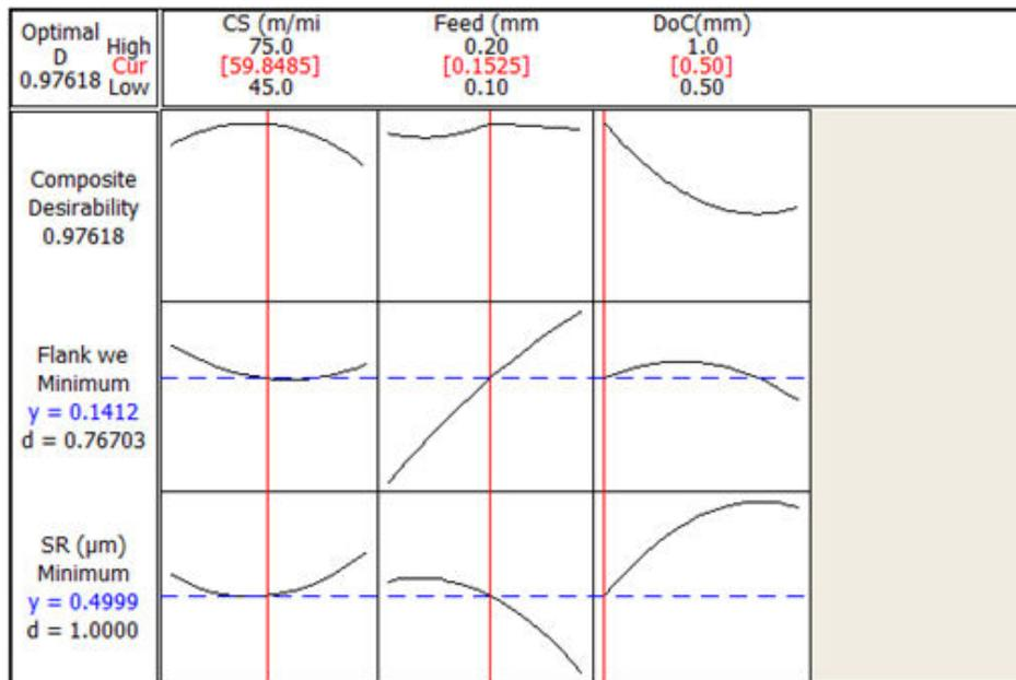
Figure 3 Response optimizer for simultaneous optimization plot.
