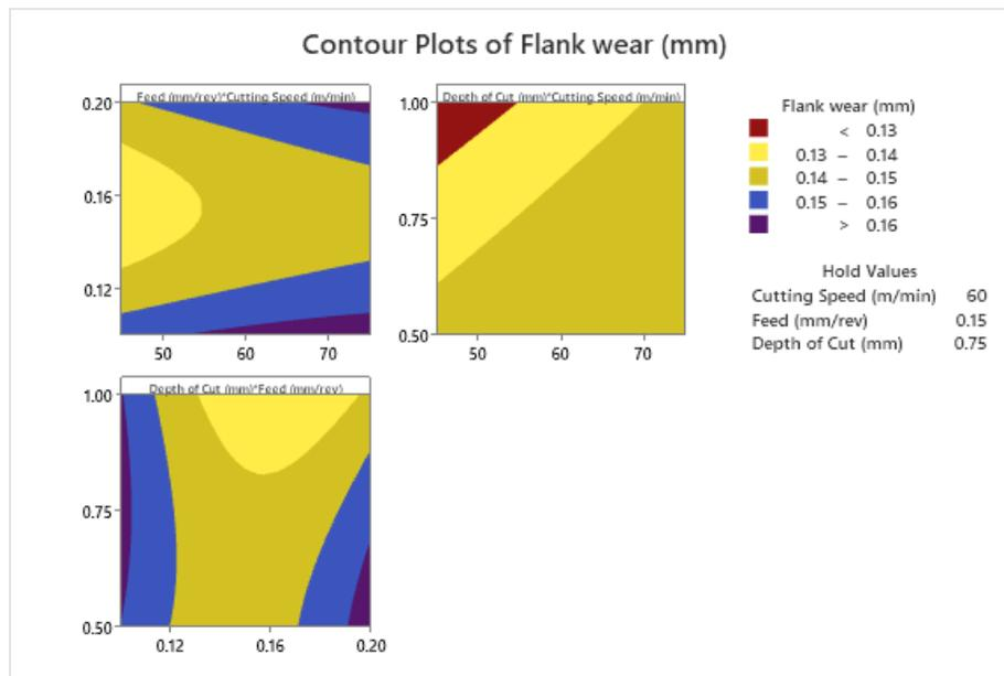
Figure 5 Contour plot for Flank wear.
