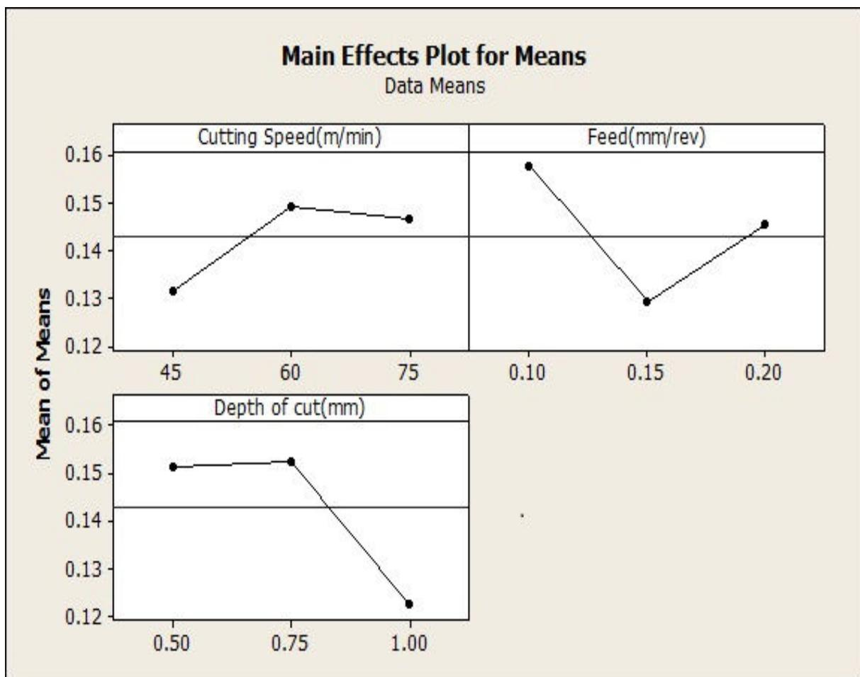
**Figure 2** Effect of cutting parameters on flank wear.
