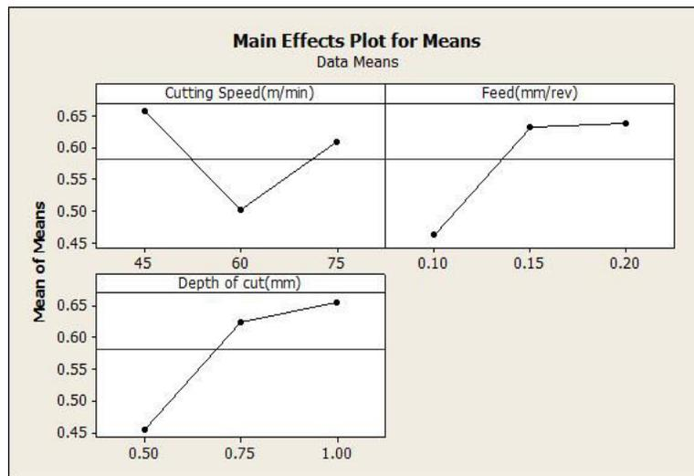
**Figure 1** Surface roughness effects on the machining parameters.
