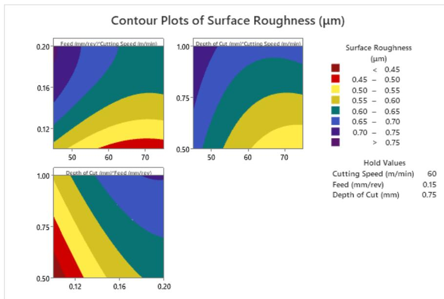
Figure 4 Contour plot for Surface roughness.
