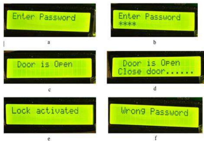
Fig. 6 Stages of operation of the digital door lock
