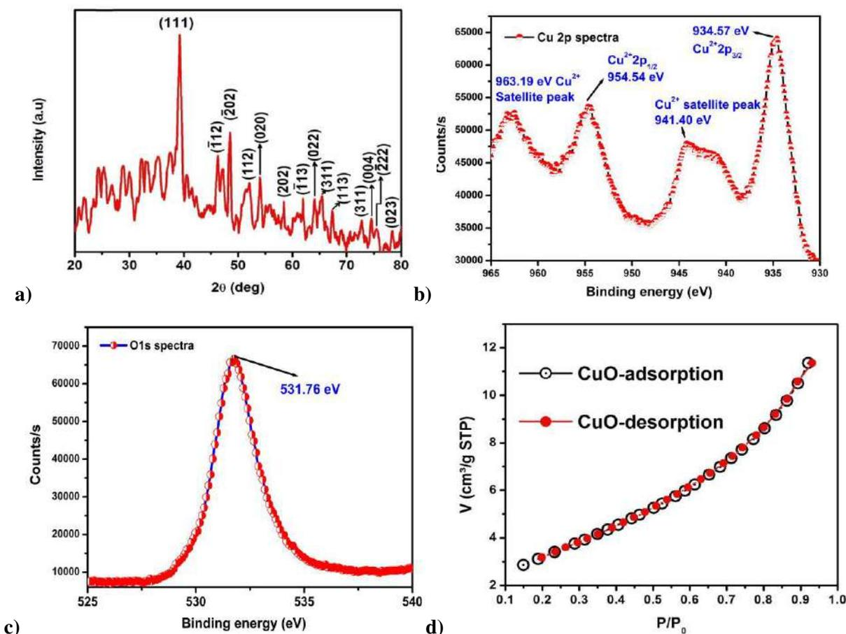
**Figure.1.** a)Structural profile b)Cu2p c)O1s core and d)BET spectrum of CuO-NPs.
