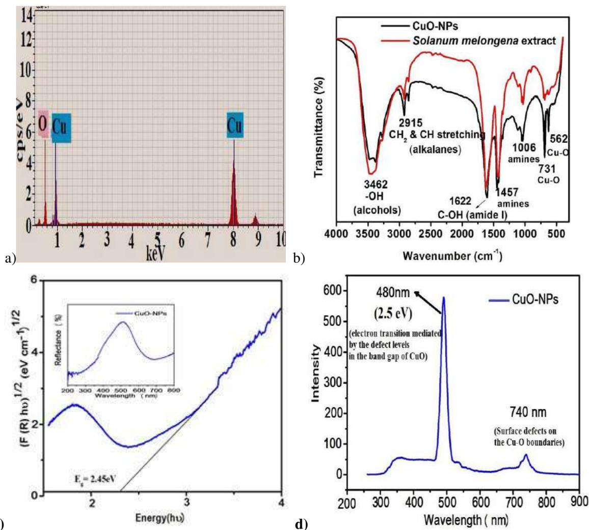
**Figure.2.a)**EDX, **b)**FTIR, **c)**Kubelka-Munke-plot (inset:absorption), and **d)** florescent spectrum of CuO-NPs.
