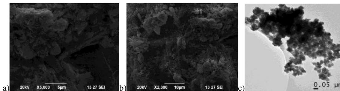
**Figure.3.** (a-b) SEM and (c) TEM images of biogenic CuO-NPs.
