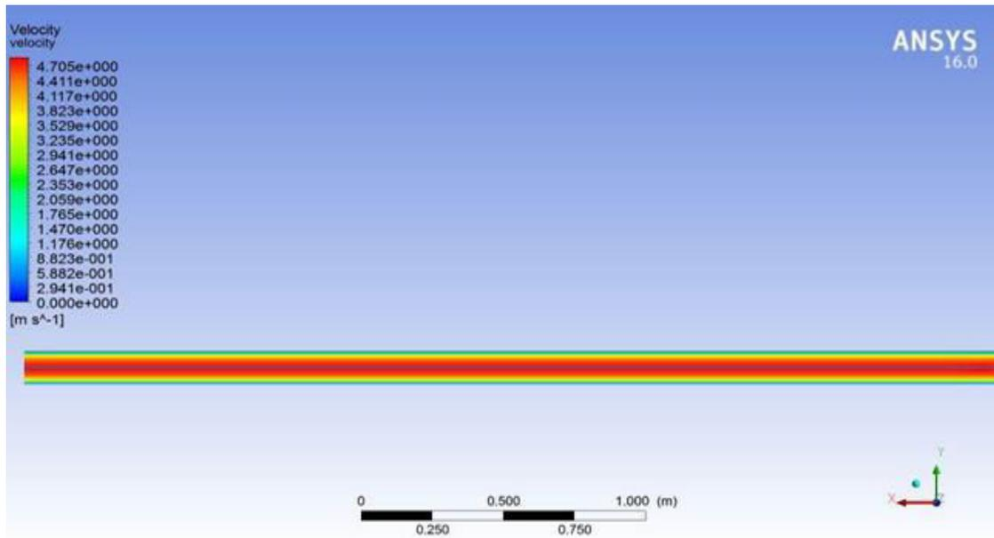
Fig: 15 Velocity profile in m/s for hot stream in NHE for constant surface area
