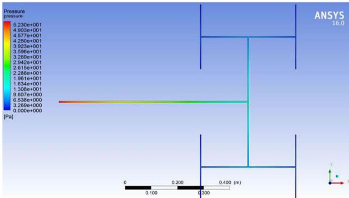
Fig: 7 Pressure profile in Pascal for hot stream in CHE
