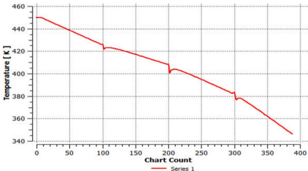
Fig: 6 variation of temperature along the chart count for hot stream in CHE
