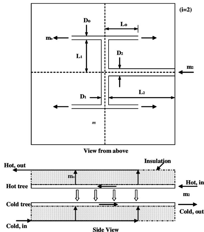
**Figure 1:** Counter flow of tree shaped streams distributed over a square area [5].
