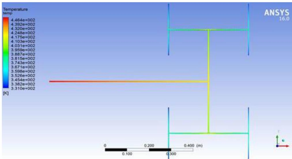
Fig: 5 Temperature profile in Kelvin for hot stream in CHE
