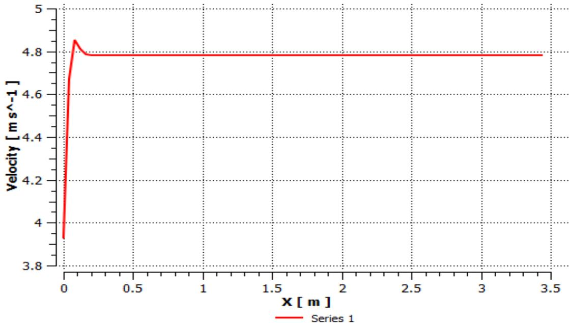
Fig: 16 Velocity variation along the NHE length for hot stream for constant surface area
