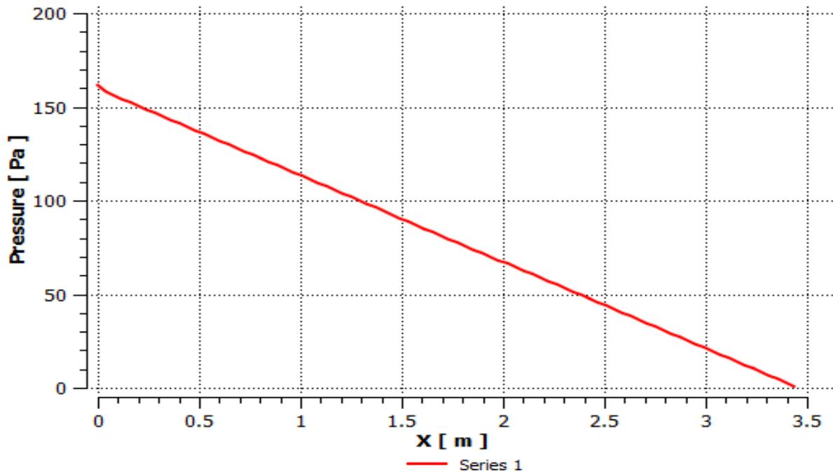
Fig: 14 variation of pressure along the length for hot stream in NHE for constant surface area
