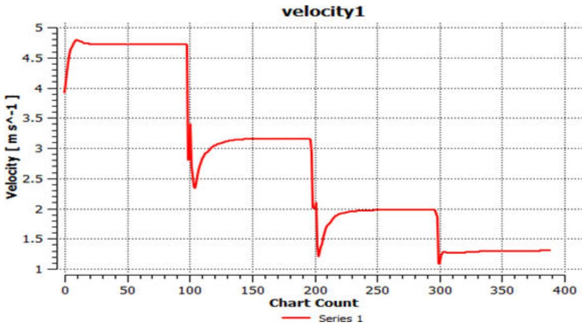
Fig: 10 variation of velocity along the chart count for hot stream in CHE
