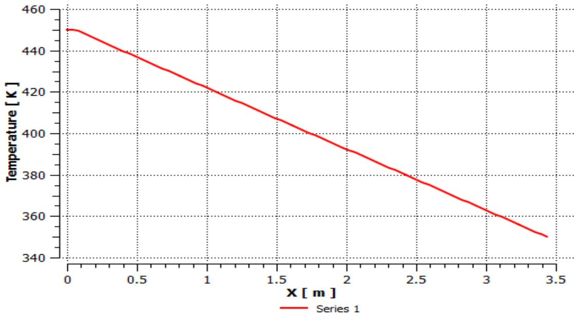
Fig: 12 Variation of temperature along length for hot stream in NHE for constant surface area
