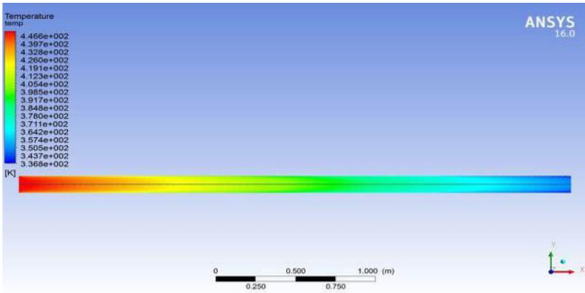
Fig: 11 temperature profile in kelvin for hot stream in NHE for constant surface area
