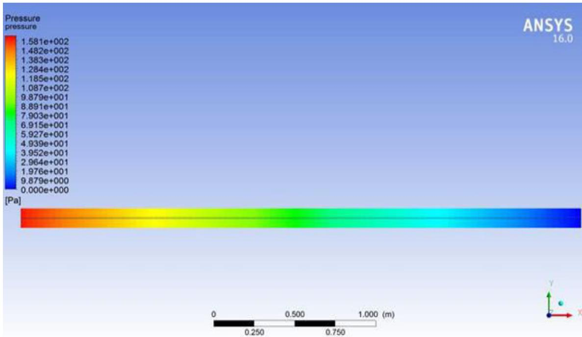
Fig: 13 Pressure profile in Pascal for hot stream in NHE for constant surface area
