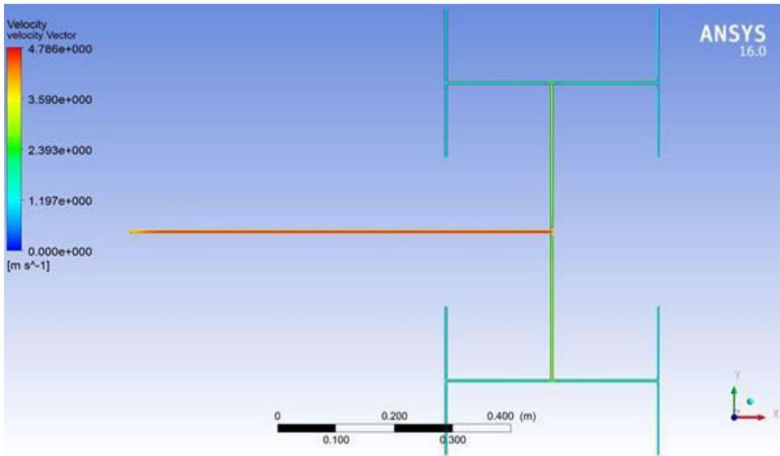
Fig: 9 Velocity profile in m/s for hot stream in CHE
