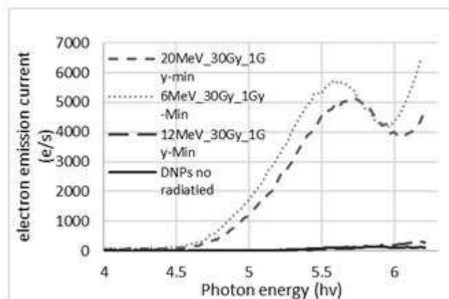
**Fig. 2:** PE spectra of tableted diamond nanoparticles tablet, dose rate of 1 Gy/min.
