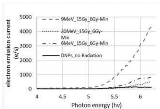
**Fig. 1:** PE spectra of tableted diamond nanoparticles tablet, dose rate of 6 Gy/min.
