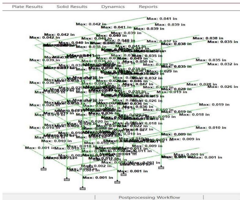
Figure Displacement of Columns
