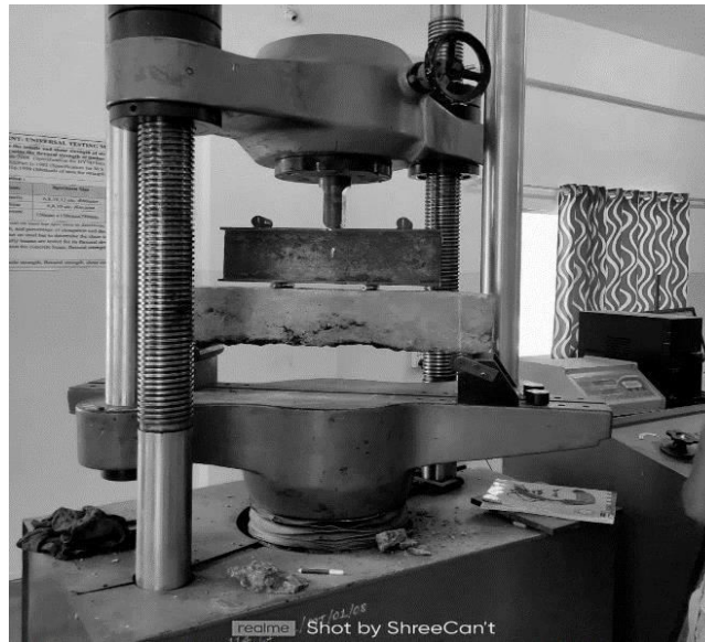
Fig 5: Flexural strength testing
