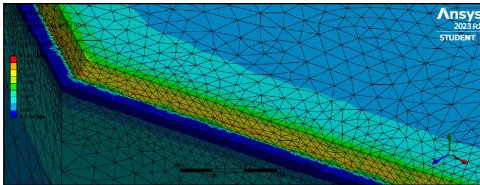
Figure 6: SPW I- Section enduring Maximum Stress
