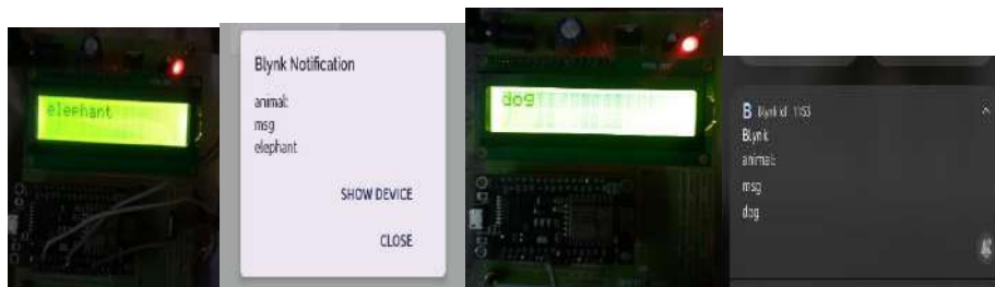
Figure 7. Outputs using LoRa and Blynk IoT
