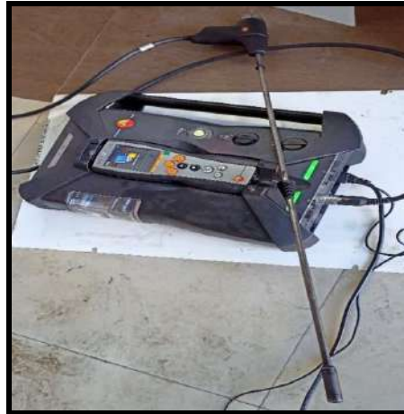
Fig. 2 Testo-350 exhaust emission gas analyser (Source: ASTU Energy Lab)
