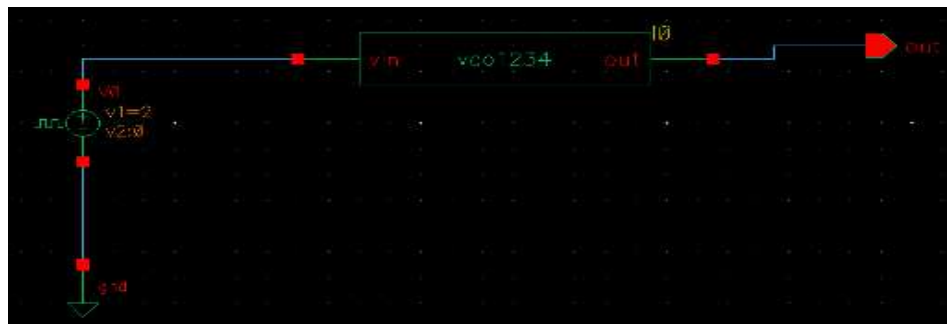
Fig 6: Test bench of VCO
