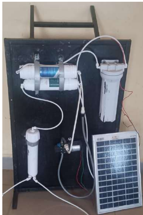
Fig 2. Water Purifier Solar Base System
