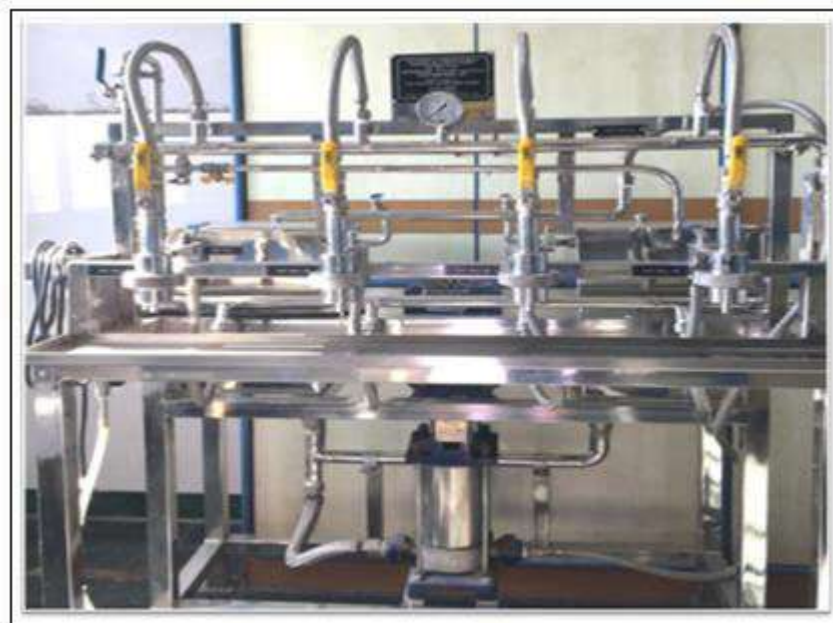
Fig. 3: Photograph of the UF Test Skid
