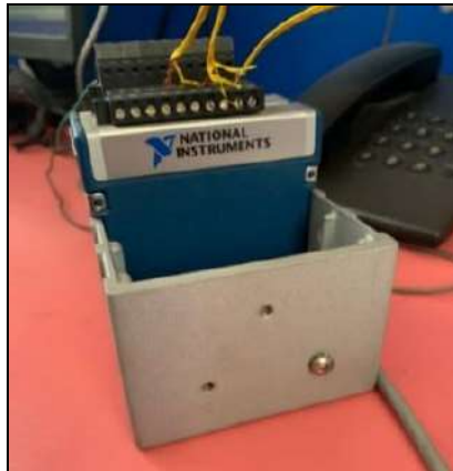
Fig. 12: Thermocouple Connected to DAQ
