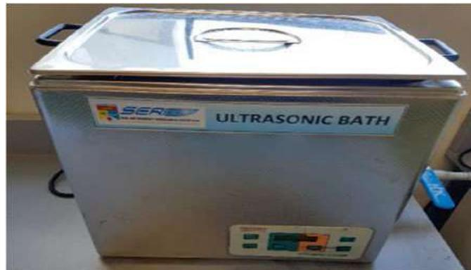
Fig. 7: Ultrasonic bath shaker [39]
