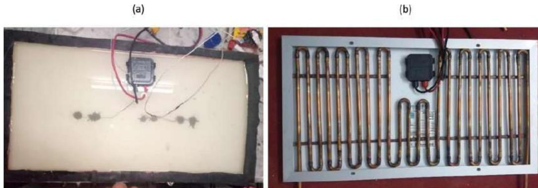
**Fig. 15**(a) Paraffin wax poured into an aluminum container as it melted; (b) a phase change material box lined with a network of serpentine copper tubes. [89]
