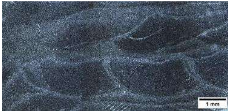
Fig. 3: Optical micrograph of 0° scanning strategy L-DED parts.
