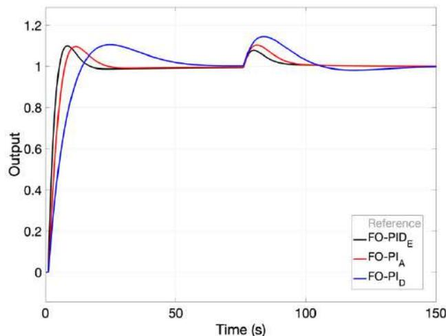
**Fig. 5.** Closed loop results obtained with the FO-PID controllers for the lag dominant process with -30% gain variation
