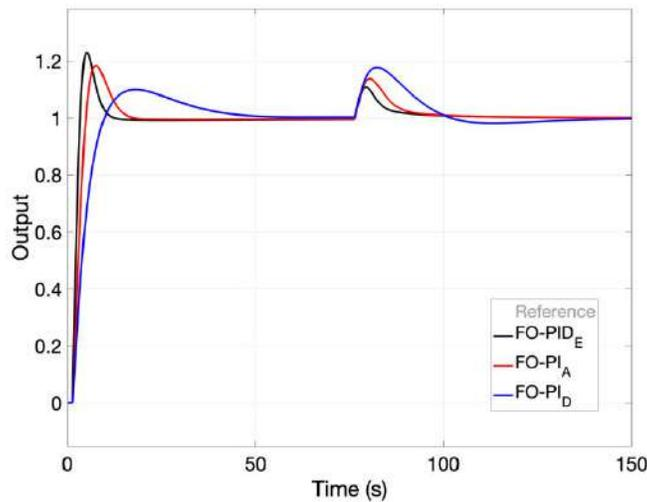
**Fig. 6.** Closed loop results obtained with the FO-PID controllers for the lag dominant process with +30% delay variation
