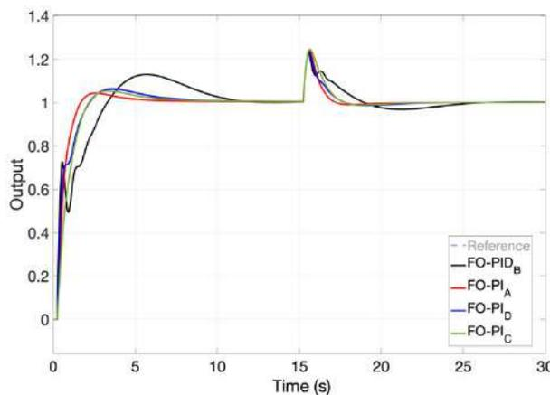
**Fig. 2.** Closed loop results obtained with the FO-PID controllers for the delay dominant process with -30% delay variation
