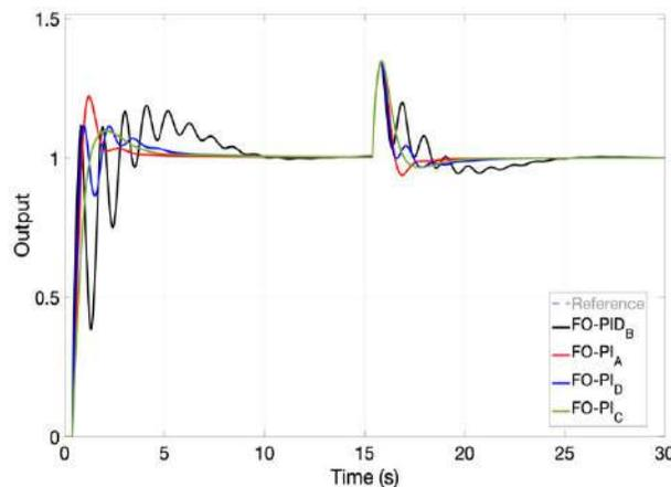
**Fig. 1.** Closed loop results obtained with the FO-PID controllers for the delay dominant process with +30% gain variation
