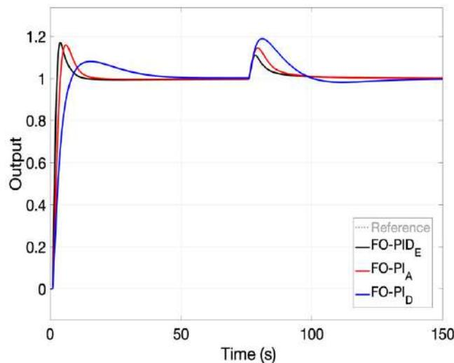
**Fig. 4.** Closed loop results obtained with the FO-PID controllers for the lag dominant process with +30% gain variation
