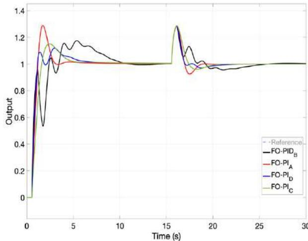
**Fig. 3.** Closed loop results obtained with the FO-PID controllers for the delay dominant process with +30% delay variation
