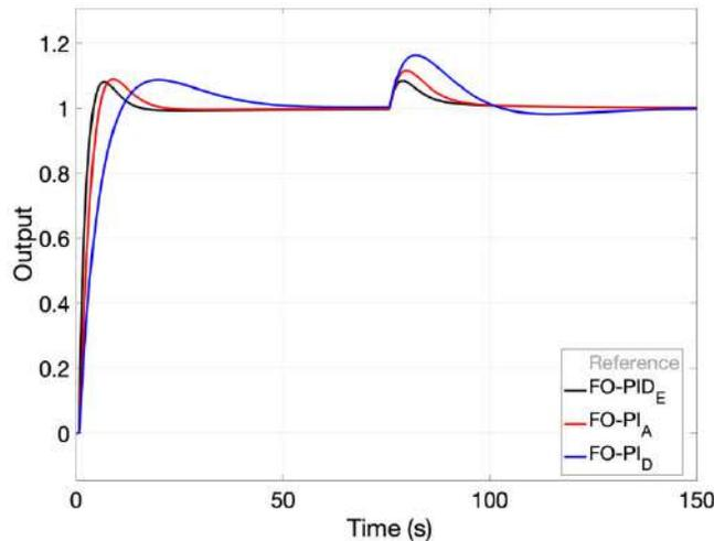
**Fig. 7.** Closed loop results obtained with the FO-PID controllers for the lag dominant process with -30% delay variation
