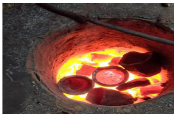
Fig. 4. Liquefying the metals in a graphite crucible in their respective ratios
