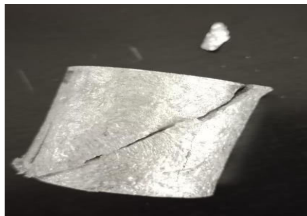
Fig. 7. Specimen after compression test
