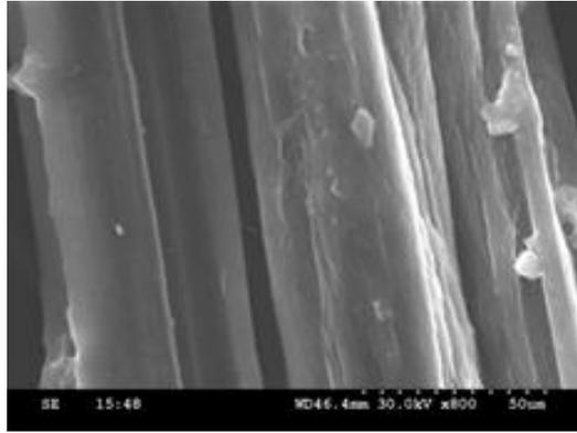
**Fig 6:** NaOH treated (boiled) specimen
