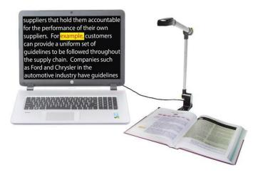
The PEARL, combined with JAWS, Fusion, or OpenBook scanning and reading software, brings blind and low vision users instant portable access to printed material with an array of human-sounding voices. The folding camera deploys in seconds to connect to your PC and snap a picture of your reading material and begins reading it aloud instantly.
