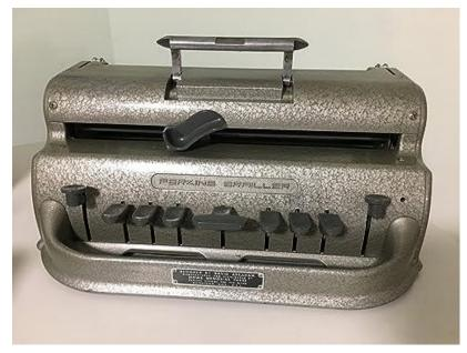
Braille typewriter is a mechanical (hand operated) writing device used for writing Braille on paper by pressing related keys.
