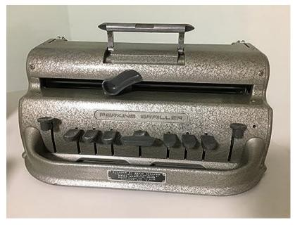
Braille typewriter is a mechanical (hand operated) writing device used for writing Braille on paper by pressing related keys.
