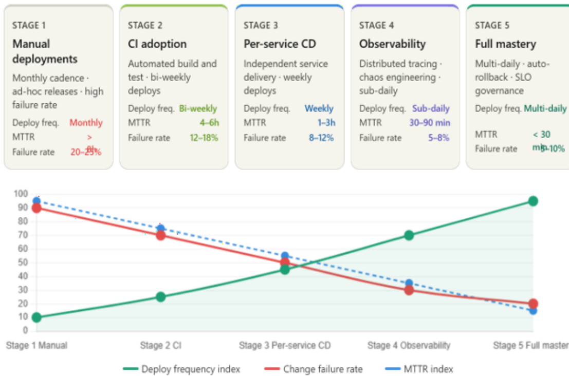
Fig. 4 — DevOps maturity progression: deployment frequency rises as failure rate and MTTR decline
