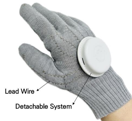
FIGURE 3 (A) SCHEMATIC OF SMART GLOVES.(B) DEVELOPED SMART GLOVES.
