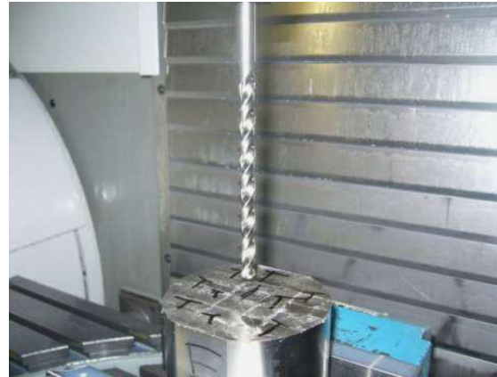
FIGURE 4. THE TITANIUM WORK PIECE WITH THE HSS DRILL BEFORE DEEP DRILLING
