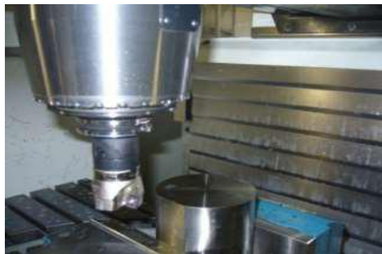
FIGURE 3. FACING OFF THE TITANIUM WORK PIECE
