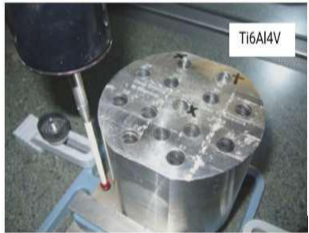
FIGURE 7. SET UP FOR MEASUREMENT OF HOLE ACCURACY
