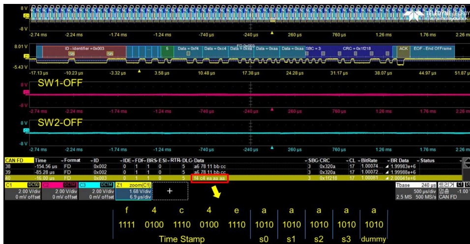
Figure 16. Cable diagnosis (normal operation)
