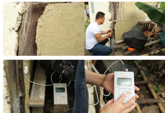
**Figure 2 OBTAINING THE HEAT TRANSFER COEFFICIENTS.**
