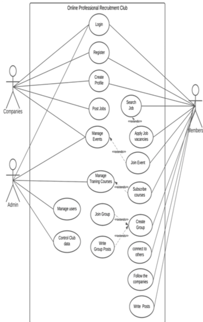
Fig. 3. Use case diagram to Modelling functional requirements
