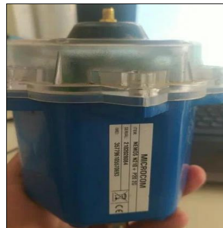
Figure 2 Datalogger NEMOS N210
