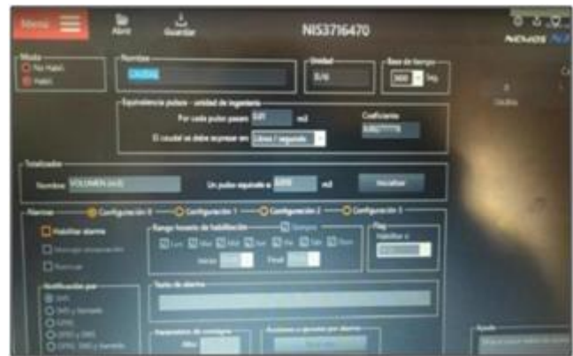
Figure 5 Configuration Of The NEMOS N210 Datalogger
