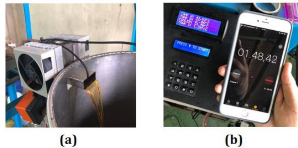
FIGURE 5 A) TESTING OF THE COOLING SYSTEM, B) MEASUREMENT OF TEMPERATURE AND TIME
