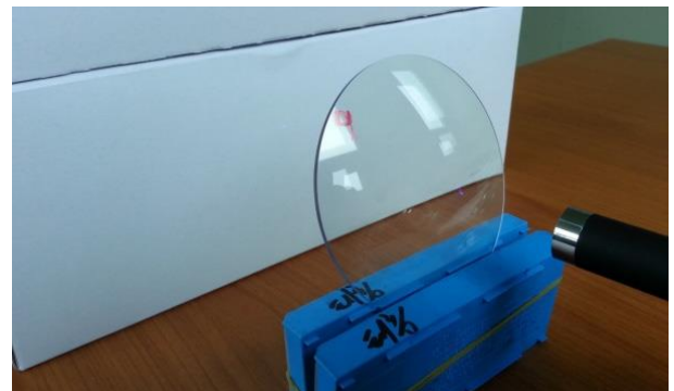
FIGURE 6 UV BLOCKING LENS, PURPLE BEAM CUT OFF
