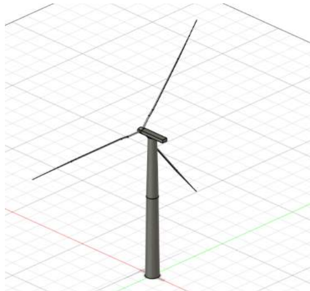
Fig. 2. Model 5 MW Horizontal axis wind turbine tower
