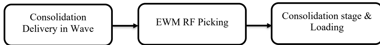
Fig. 1. Outbound processing: Consolidation of deliveries in wave picking, RF picking, and consolidation into staged/docked and loaded shipments.
