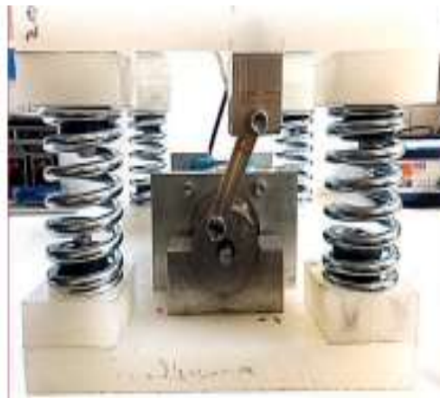
Fig. 6: The fabricated prototype (a) R-P mechanism with a Top Plate 1 , Rack 2 , Pinion and clutch 3 , Gearbox 4 , Generator 5 , Pinion Support 6 , Support 7 , Compression Spring 8 . (b) L-GE mechanism with Electrical Coil 9 , Set of Magnets 10 , Rod 11 .
