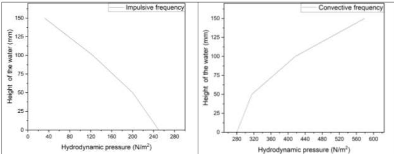
**Fig. 10: Hydrodynamic pressure distribution - Model-3**
