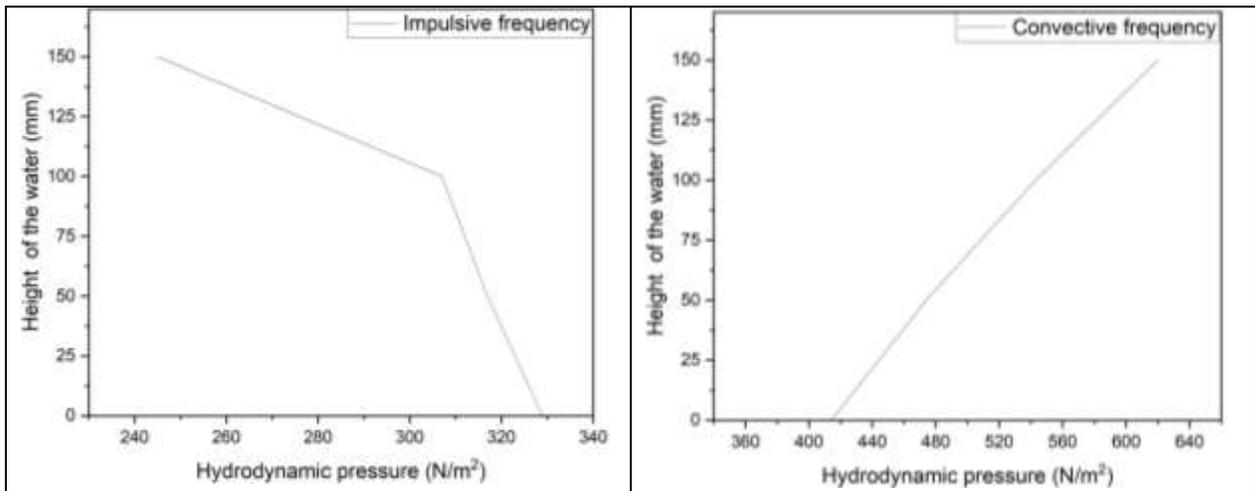
**Fig.8: Hydrodynamic pressure distribution - Model-1**
