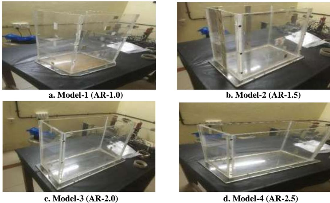
**Fig. 5: Acrylic models used in the experimental study**
