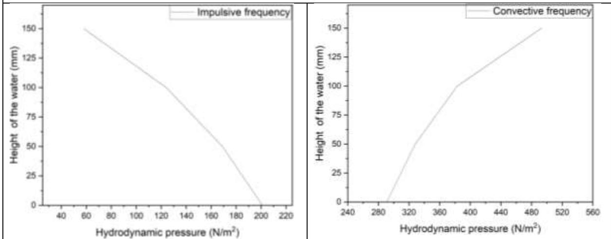
**Fig. 11: Hydrodynamic pressure distribution - Model-4**
