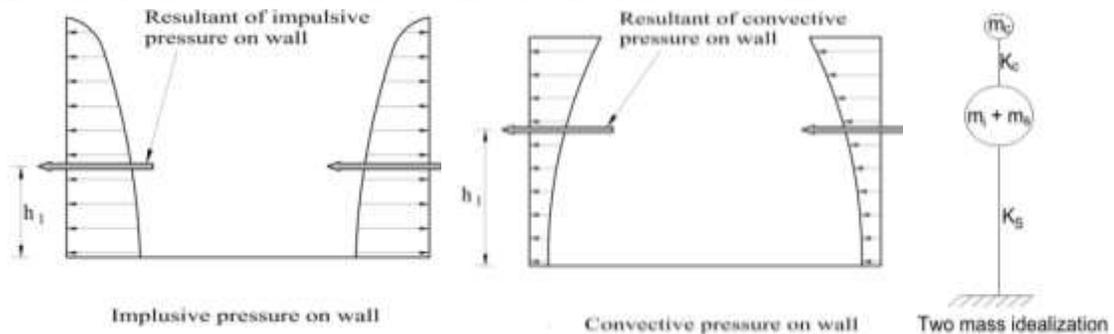
**Fig. 1: Description of hydrodynamic pressure distribution on tank wall and two mass idealisation [6]**
