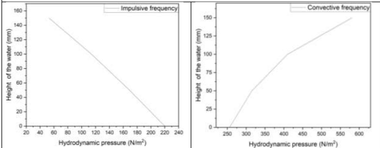
**Fig.9: Hydrodynamic pressure distribution - Model-2**
