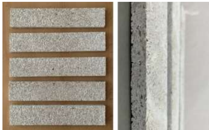
Fig. 2 The appearance of the cut samples for determining mechanical properties
